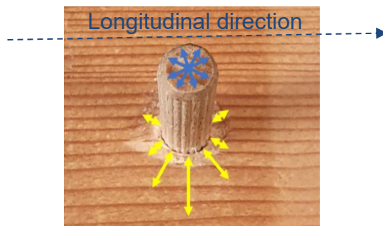
Figure 1. Wood-wood connections with the corresponding swelling/shrinking directions
