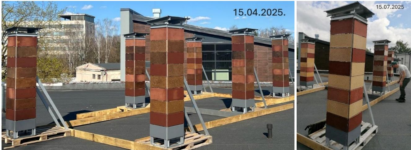
Figure 2. Long-term natural weathering test of produced panels.
