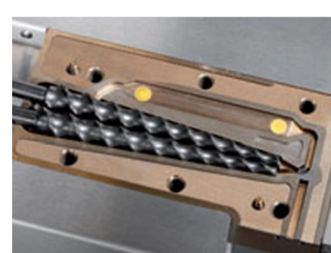
Co- and counter-rotating twin screws
