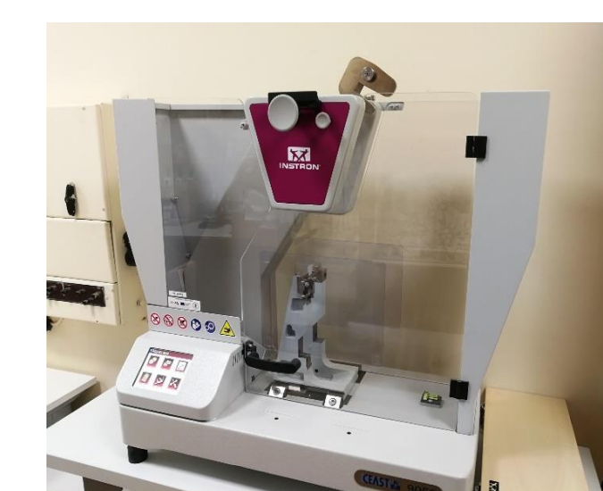
Pendulum Impact Testing Machine “Instron CEAST 9050”
