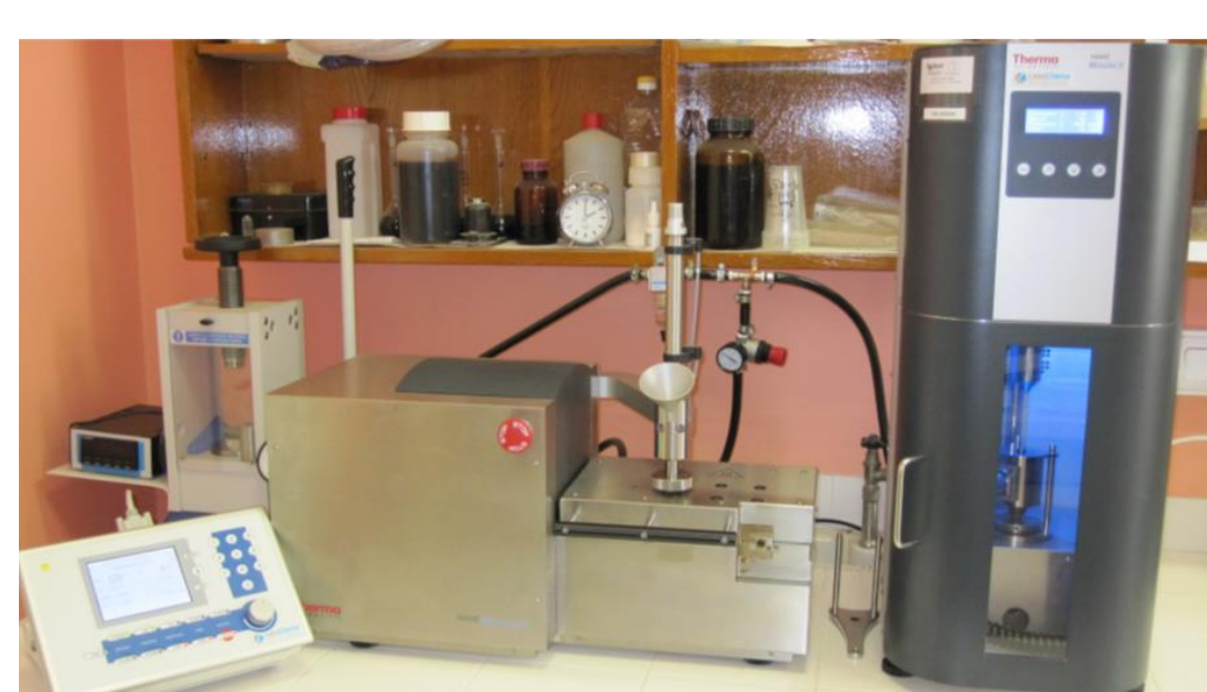
Laboratory equipment for wood-plastic composite processing HAAKE MiniLab II and MiniJet II, (Thermo Scientific)
