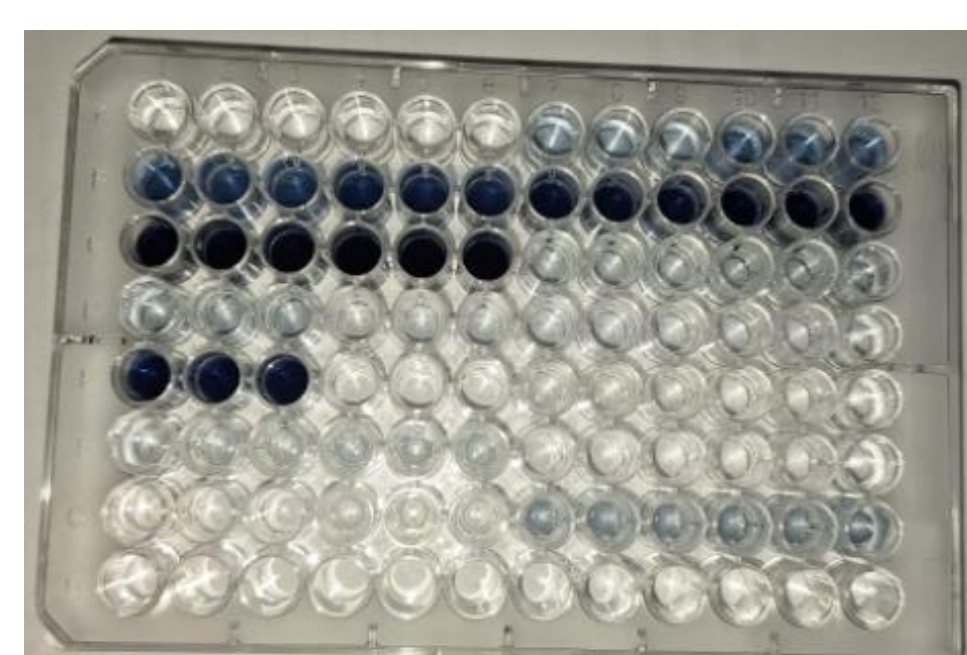
Fig. 2. Bark extracts TPC analysis using optimized Folin-Ciocalteu method on 96-well microplate
